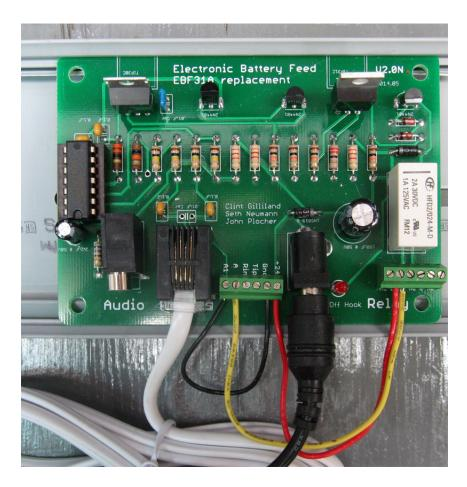
Figure 3 - Off Hook Indicator Wiring
